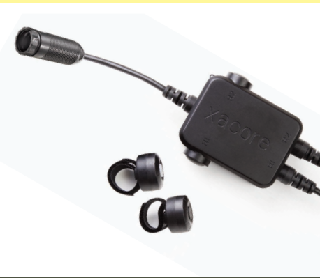
THREE RADIO VERSION W/ x-62000 HEADSET MODE & VOLUME CONTROL, WIRELESS PTTs AND ICS/INTERCOM BAIL-OUT CORD INPUT (3 POSITION TOGGLE SWITCH)
