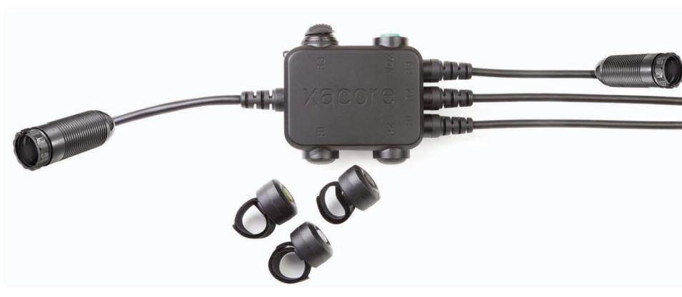
THREE RADIO VERSION W/ x-62000 HEADSET MODE & VOLUME CONTROL, WIRELESS PTTs AND ICS/INTERCOM BAIL-OUT CORD INPUT (3 POSITION TOGGLE SWITCH)
